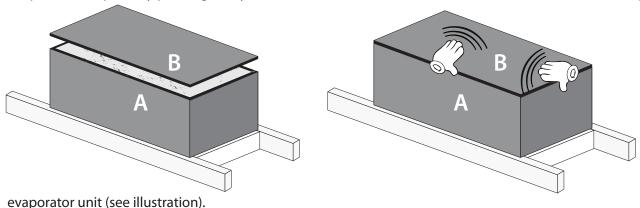
If needed, trim excess insulation around all edges.
