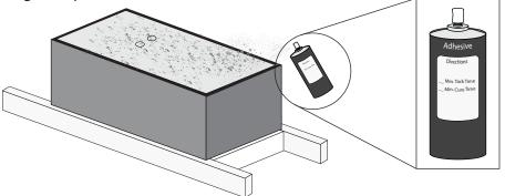
8. Set piece (B) in place by pressing firmly on all surfaces of the insulation that come in contact with the top of the evaporator unit (see illustration).
