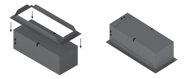
4. Secure the unit's mounting bracket to the opening using the twelve (12) supplied 2<sup>1</sup>/<sub>2</sub>" Phillips-head screws.
