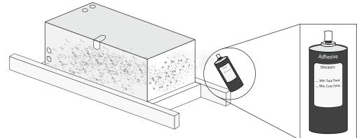
3. Wrap insulation piece (A) around the sides of the evaporator unit. Make sure the bottom edge of the insulation is flush with the top edge of the mounting bracket (see illustration).
