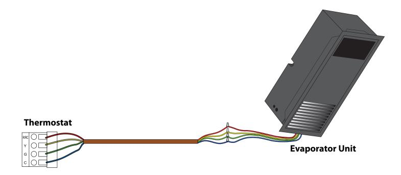
**NOTE:** To ensure correct system operation, the 24V thermostat must be placed inside the wine cellar, preferably in a central location away from any airflow.
