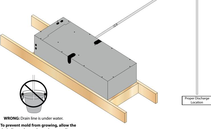
drain line to hang above the water line.
