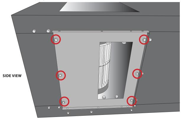
6. Reinstall the previously removed side panel in the old blower location using screws removed earlier. Use a low torque setting on the drill to avoid stripping the holes.
