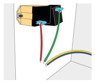
4. Replace the center access panel and re-secure using the six (6) screws removed earlier. Install a black strain relief around the 18-5 thermostat wire going into the unit as shown.
