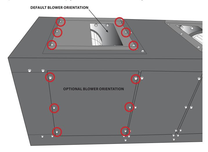
3. To reorient the blower(s), first remove the screws securing the supply panels on the top and preferred side of the unit (as shown above). Remove the panels.
