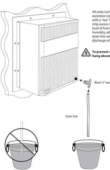
All units come with a drain line for additional removal of excessive condensate. It is mandatory to install the drain line with a "tee" fitting. During operation, the cooling unit will strip excess water from the air in order to maintain the proper level of humidity within the cellar. However, in extreme humidity, additional condensate will be removed. The drain line will prevent overflow and leaking by allowing for discharge of the additional condensate.
