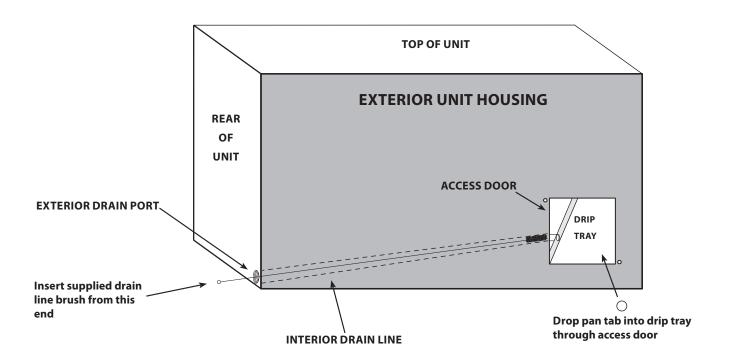
Pan tabs kill bacteria and related odors, remove sludge and scale, and help to prevent water damage caused by condensate overflow. They are non-corrosive and easy to install. Simply use the access door to drop a pan tab into the drip tray every six weeks.
