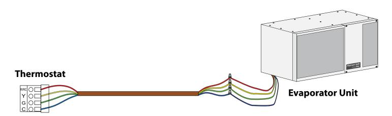
**NOTE:** To ensure correct system operation, the 24V thermostat must be placed inside the wine cellar, preferably in a central location away from any airflow.
