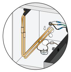
11. Remove the line set caps. Route the  $\frac{3}{6}$ " suction line and  $\frac{1}{4}$ " liquid line into the unit and braze.
