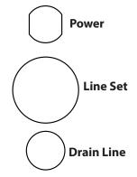
6. Depending on the desired installation, remove the rear or bottom knockouts for the line set, drain line, and power cord.
